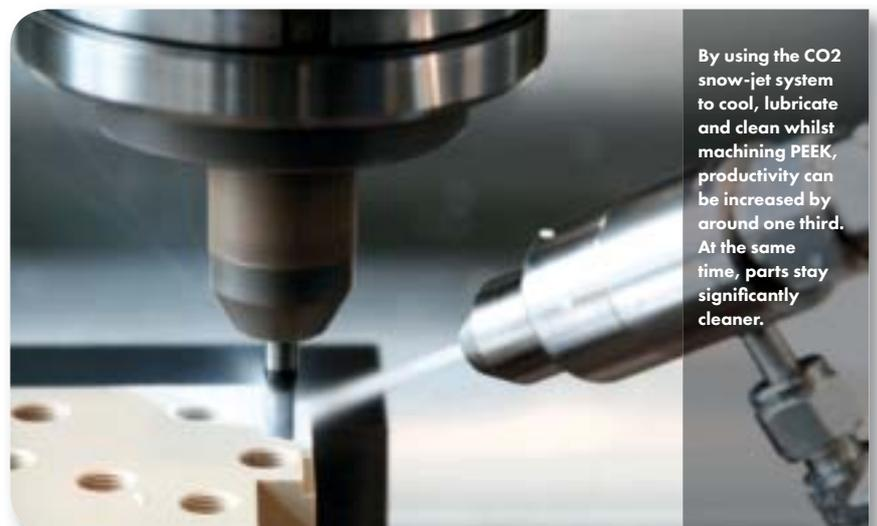
By using the CO<sub>2</sub> snow-jet system to cool, lubricate and clean whilst machining PEEK, productivity can be increased by around one third. At the same time, parts stay significantly cleaner.
